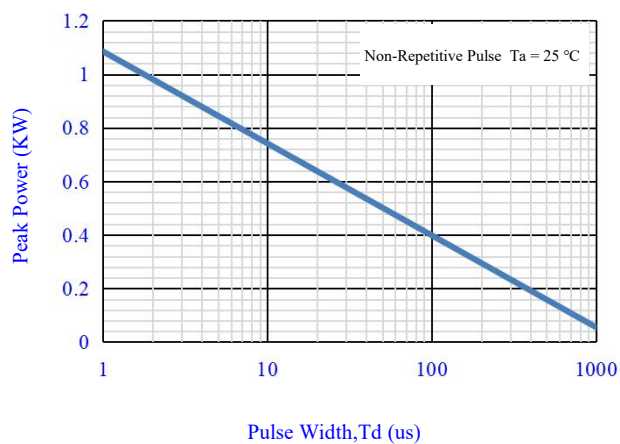
Fig.3-Peak Pulse Power Rating Curve
